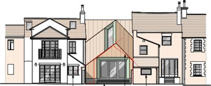
PROPOSED REAR ( WEST ) ELEVATION Angle subtended by existing roof retained for daylight. Flood valves behind grille positioned as agreed by the Environment. Outline of existing building. Angle subtended by existing roof retained for daylight.
